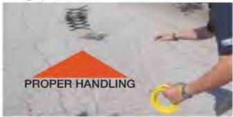
The cord is released off the loop as the system is deployed. The winder can be attached to the right or left hand eyelet.
