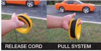
The loop winder has a beveled side and allows rope to be released when it is twisted towards traffic. When the loop is spun back, it catches the cord and allows you to pull the system in place or retrieve the system from traffic.
