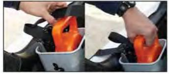
To access the system, unhook the strap. Then Remove the Winder from the Holster with your non dominant hand.
