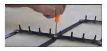
Tighten the screws just enough to prevent the washer from turning. Do Not Over Tighten!
