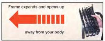
The other side of the Spike-Strip frame is loose and is the side that expands and opens up away from your body and onto the roadway.
