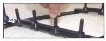
The Spike-Devil uses a cartridge, the top half of the Spike is covered with a cap / seal. You can cover the bottom portion of the cap with Silicon, and the end of the exposed spike tip with water. Place the exposed portion into the Spike Strip receiver hole, rotate until the slot on the spike aligns with the length of the Strip. Press the cartridge down into the hole.
