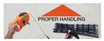
The cord reel is attached to the Spike-Strip frame Notice the crank is facing towards the officer and unhooked to allow slack and deployment.
